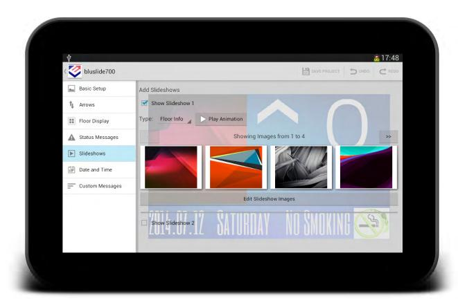
The application can run on any Android smartphones or tablets. After you connect to the elevator display via Bluetooth or Wi-Fi, it is possible to access the display's menu, set the clock or upload a completely new design. You can also create these designs from scratch, or modify an existing one. The result can be shared with colleagues, or naturally it can go directly to the elevator.
